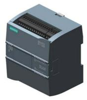
SIMATIC S7-1200, CPU 1212C, compact CPU, AC/DC/relay, onboard I/O: 8 DI 24 V DC; 6 DO relay 2 A; 2 AI 0-10 V DC, Power supply: AC 85-264 V AC at 47-63 Hz, Program/data memory 50 KB
